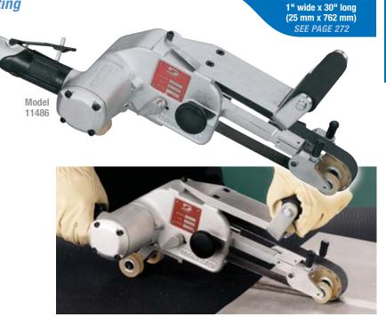
Place 11486 Dynabelter handle at 45° angle from belt housing to increase grinding pressure. Pull tool toward operator for faster material removal.
