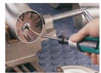
3" Eyelet Sanding Star easily enters pipe elbow using 7" long flexible mandrel.
