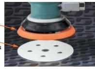
Loop material attaches to standard — Hook-Face sanding pad
